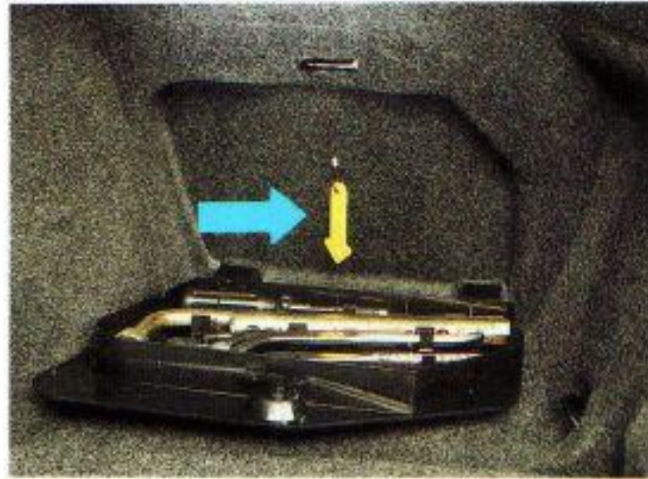
Cord for emergency opening of fuel filler flap SG1240
