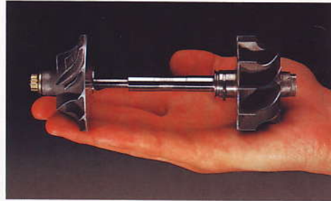
A turbine wheel—the foundation of turbo power.
